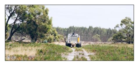
Seismic surveys require a mobile energy source to send sound waves deep into the ground and an array of recording devices planted in the ground in a pattern around the energy source. As the sound waves travel downward, they are partly reflected back to the surface at the boundaries between layers of different rock type.
