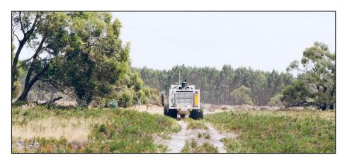
Victoria's gas supply has been safely sourced for over forty years through the use of geophysical seismic surveys to locate gas reservoirs. Virtually all gas exploration wells, onshore and offshore, are drilled on locations that have been identified by seismic survey data. Scientifically based seismic surveys are undertaken by contractors using equipment designed specifically for these operations.
